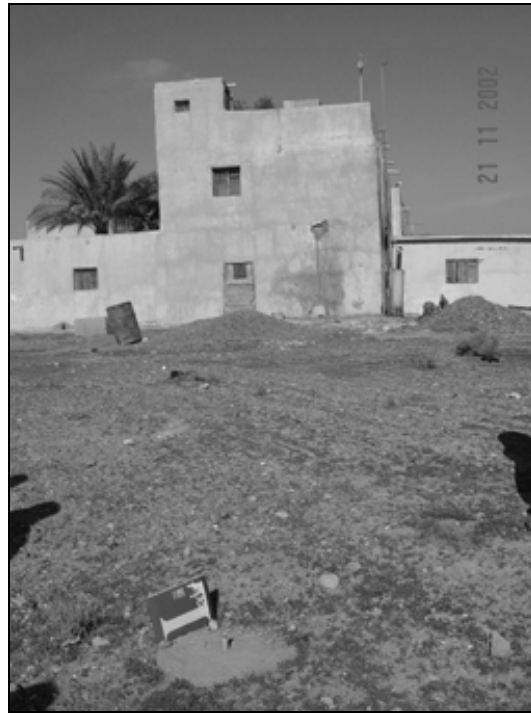
Pl. 3.1: Ashur. Benchmark indicating the maximum flooding level of the Makhool Dam reservoir: 155,67 m above sea level Location: c. 20 m south of the house of the expedition (Photograph: A. Hausleiter)
