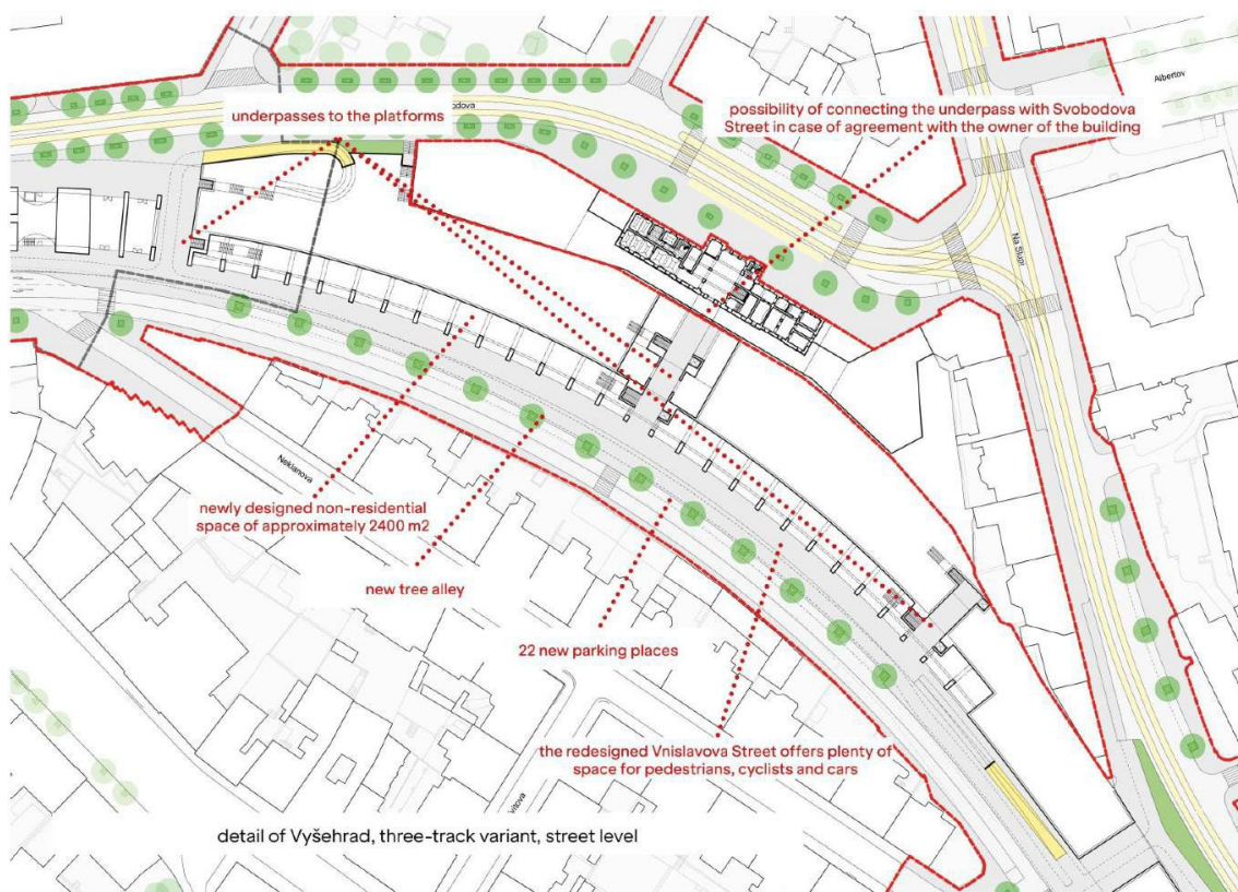
Fig. 24 Detail: Alternative three-track scheme, street level, Vyšehrad.
