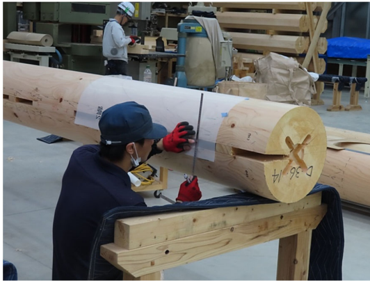
The large timber elements are mechanically milled and carefully measured. © C.Forbes 2023
