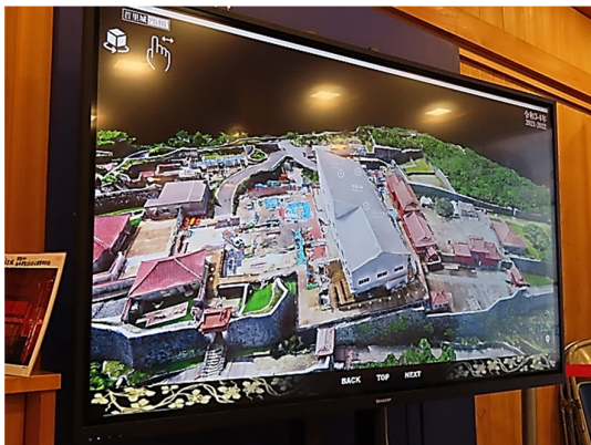
Video image showing the workshop built on a raised platform over the central courtyard to ensure minimal impact on the archaeology below. © C.Forbes 2023
