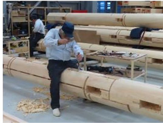
Joints are finished by hand to ensure a tight fit. Carvings will also be completed by hand. © C.Forbes 2023
