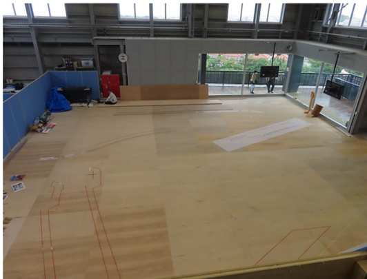
A large space is used for full scale drafting of individual elements for reconstruction. Large windows in the workshop walls allow visitors to see the work in progress. © C.Forbes 2023
