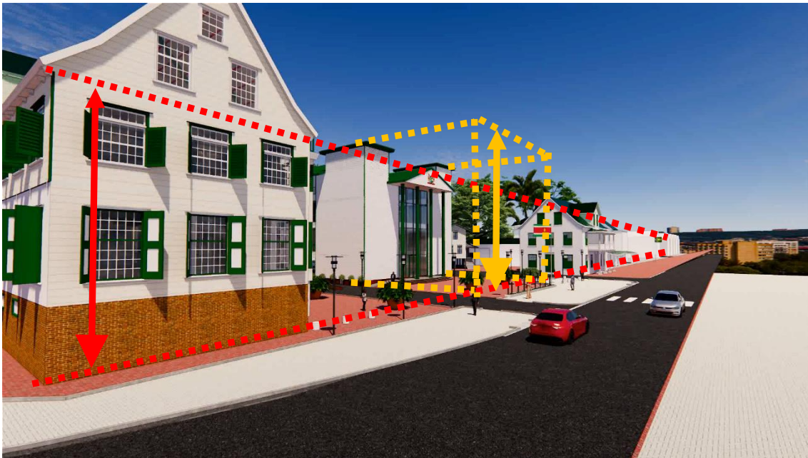
Photo 52: Analysis of the height of the proposed new building (yellow) as projected without its setback and within the context of the average height/proportion of most buildings (red) along Grote Combeweg . Rendering by de Architecten studio.
