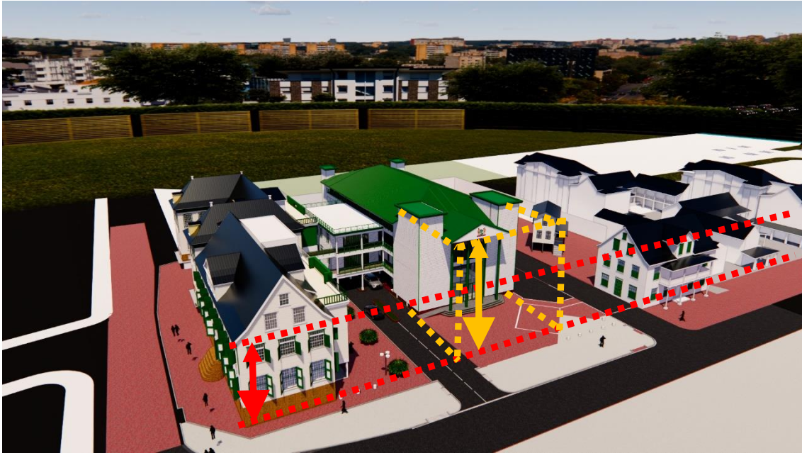
Photo 51: Analysis of the height of the proposed new building (yellow) as projected without its setback and within the context of the average height/proportion of most buildings (red) along Grote Combeweg . Rendering by de Architecten studio.
