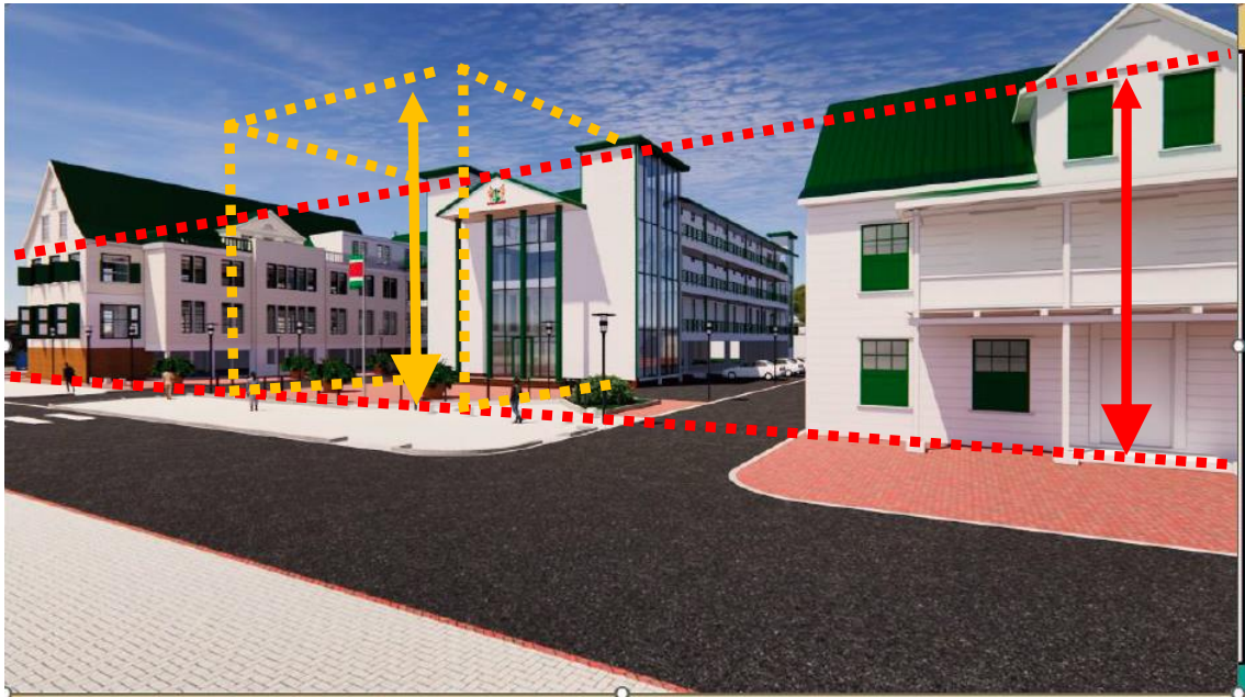
Photo 53: Analysis of the height of the proposed new building (yellow) as projected without its setback and within the context of the average height/proportion of most buildings (red) along Grote Combeweg . Rendering by de Architecten studio.
