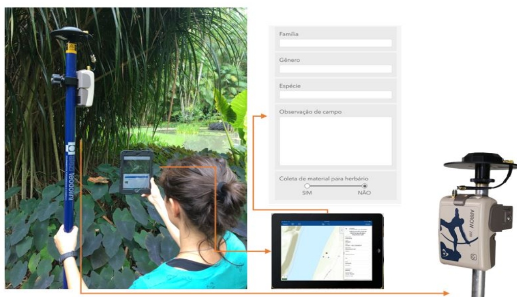
Point collection with GNSS and below, ArcGIS interface with maps of the area associated with the collection points.
