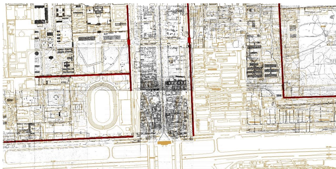
Fig. 3-6. Topographic map showing the overlapping positions of the Yongdingmen Gate Tower in 1954 (black lines) and 2018 (brown lines)
