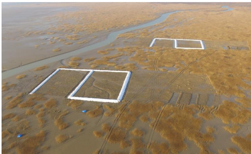
Figure 20 Semi- and Fully-Enclosure Techniques for Spartina alterniflora Loisel. Control (Source: Feasibility Study Report on Comprehensive Coastal Wetland Restoration Project of Shandong Yellow River Delta National Nature Reserve)
