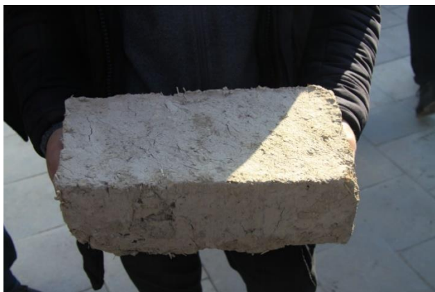
FIGURE 34: (ABOVE) MAKING MUD -STRAW BRICKS FOR RE-USE IN THE REPAIR WORKS
