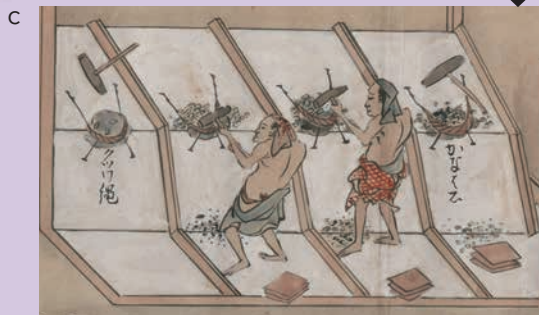
c Crushing ores: Place the ores on the pounding stones and crush them finely with hammers.
