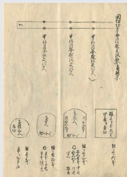
● Figure 60 Management of excavation progress (above: standard points) and cross sections of mining tunnels (below)
