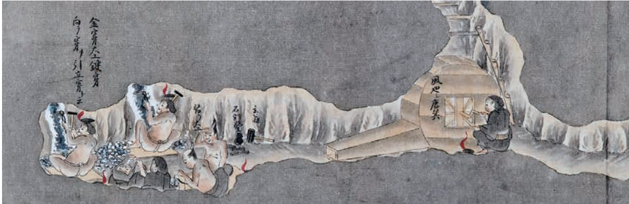
● Figure 27 Air ventilation using winnowing fan “Sado no kuni kinginzan shikioka kasegikata no zu” (Picture of mining method in Sado gold and silver mines (inside and outside)) [Property of Niigata Prefectural Museum of History]
