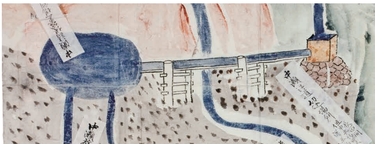
● Figure 13 The picture of “Toi” (wooden sluice to cross over streams and valleys) “Nishimikawa Sakinzan Suirō zu” (Drawing map depicting the location of waterways in the Nishimikawa Placer Gold Mine)
