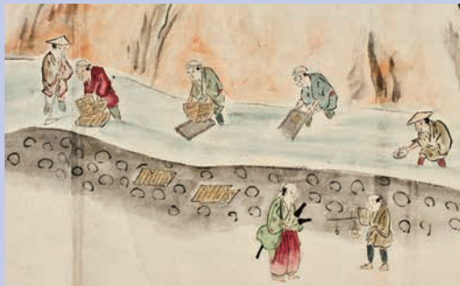
[f] Put dirt gathered in processes d and e on Yuriita, panning board and collect placer gold with gravity concentration.
