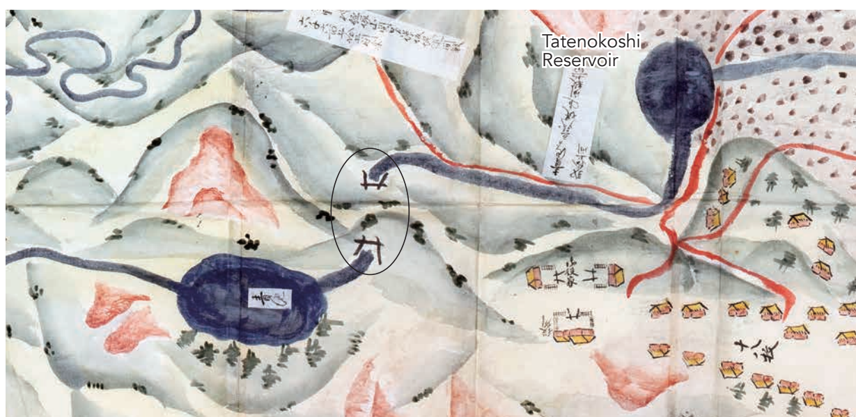
● Figure 14 Tunnel called “Kirinuki” (headrace in the Tatenokoshi-yama Site) “Nishimikawa Sakinzan Gofushin Tsukamatsuru Sumibiki” (Drawing map regarding public works by the government in the Nishimikawa Placer Gold Mine)
