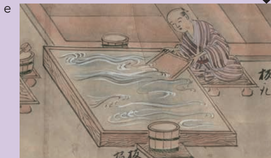
e Gravity concentration: Put the sand-like ore in a water tank and collect heavier gold and silver with panning board.
