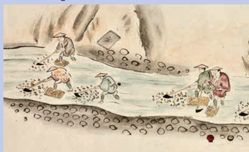
[d] Gather sand collected on the bottom of the race on Nekoda mat, (wash away unwanted dirt with the water force), and collect the minute sand by sifting through the mesh of the Nekoda mat.
