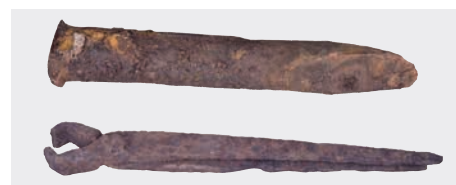
● Photo 3 Cold chisel (above) "Ueda-bashi" (below) pincer-like tools for holding the cold chisels
