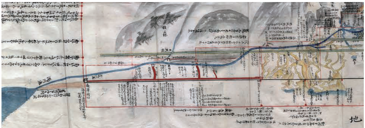
● Figure 29 Cross-sectional view of the Minamizawa Drainage Tunnel Site “Sashu Aikawa soginzan shikioka kogefurikane ezu” (Sado Aikawa surveying cross-sectional map:1696) [Property of Golden Sado Inc.]
