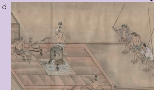
d Grinding: Grind the crushed ores with stone mill.
