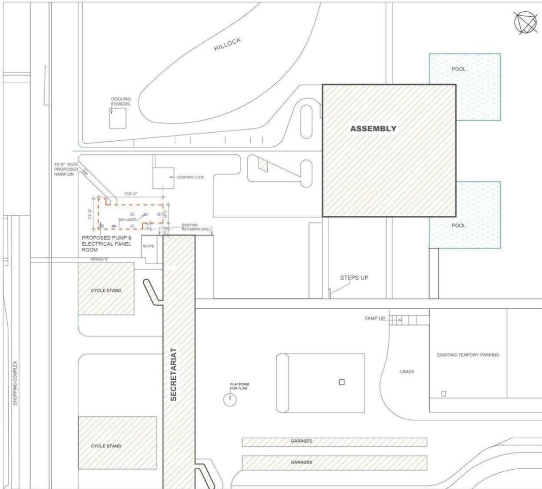
Image 34: Location of Proposed Site for AC plant Room with Electric Substation and Cooling tower
