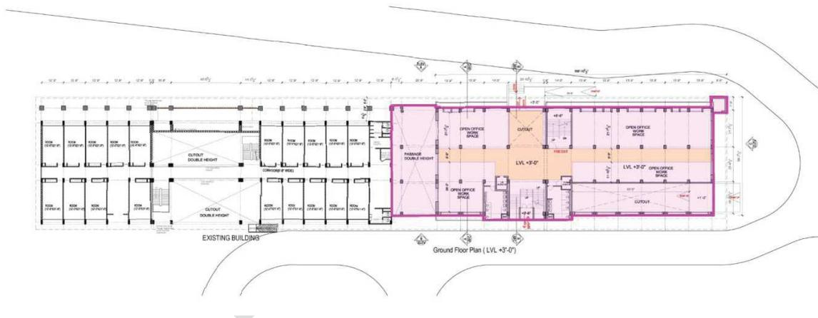
Image 25: Proposed Plan of Block-3 with red indicating the modification/extension to the existing building; Green indicates the new block Ground Floor © Satnam Namita and Associates
