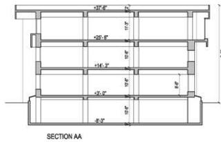
Image 27: Proposed section AA of Block-3 © Satnam Namita and Associates
