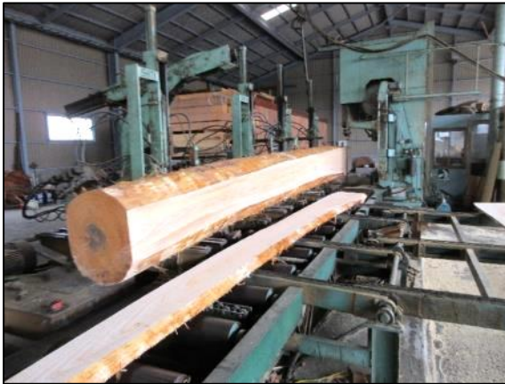
Sawing of procured lumbers
