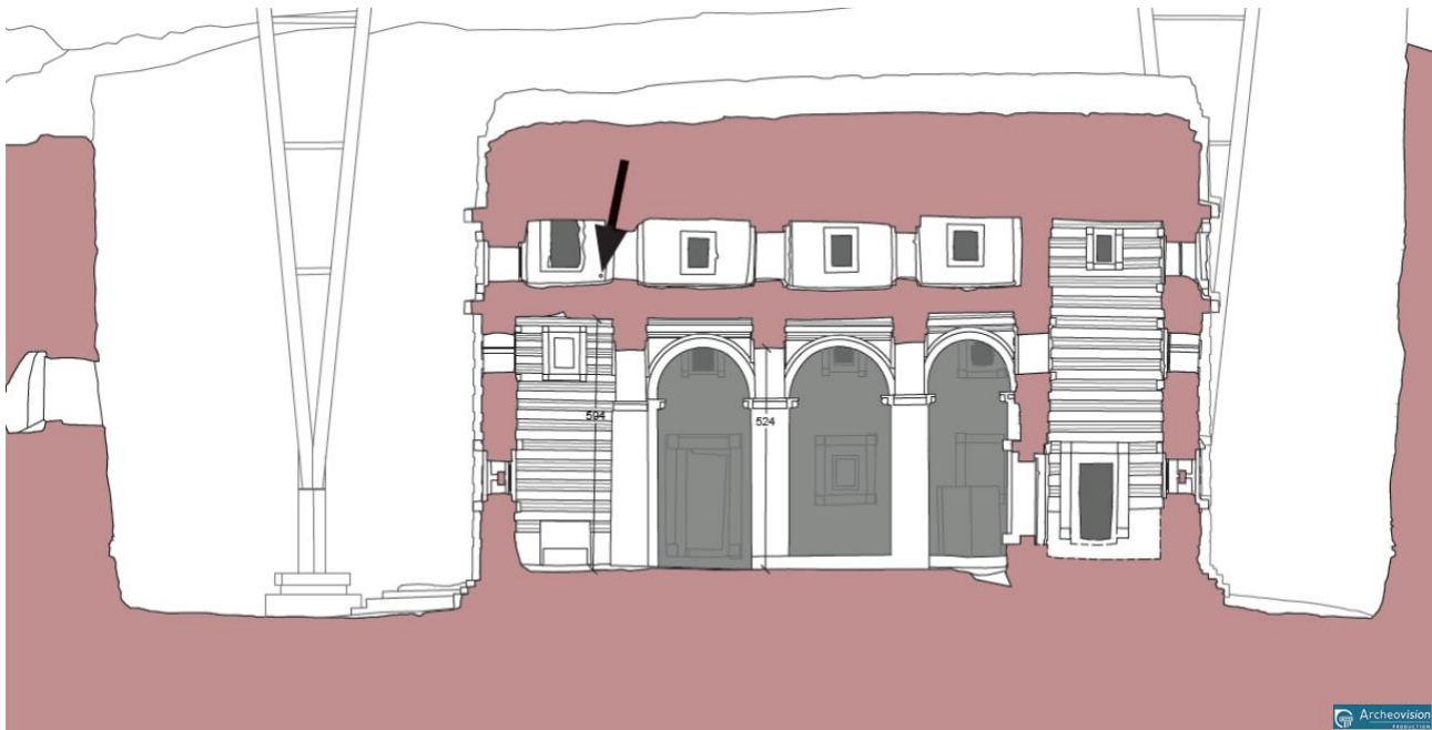
Figure 98: Biete Amanuel – Presence of the transversal tie rod in the western gallery
