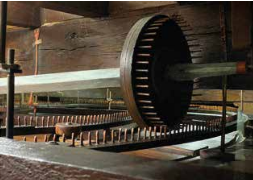
48. The mechanism of wooden hoops and discs, fitted with approximately six thousand iron pins that functions as a gear.
