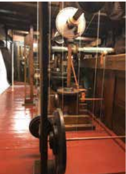
49. 50. 51. The pendulum clock with nine weights that powers the mechanism.
