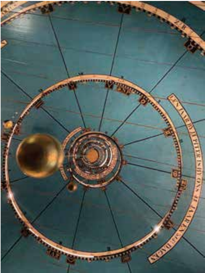
52. 53. 54. The Prussian blue and gold painted ceiling along which the planets move, including the spheres of the sun and the earth, attached to cords, and in which five dials are fitted.
