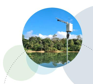
A water quality monitoring micro station at Nash's Crossing in the Lower Herbert River which monitors river levels and concentrations of nitrate and sediment in near real time: © The State of Queensland
