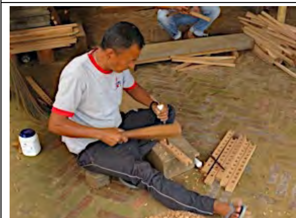
Carpenter making lattice screens for sattal
