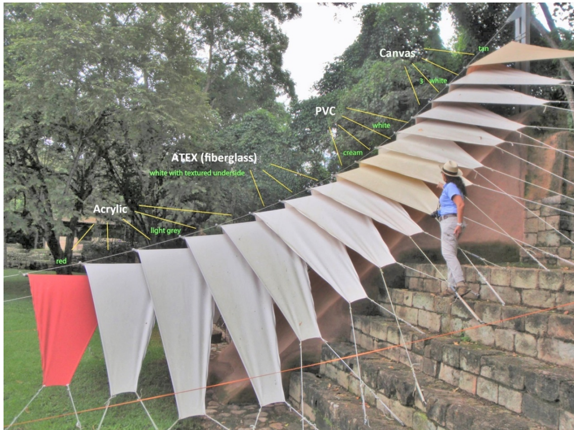
Figure 6: Prototype of the “Cascading Sails” protective structure for the Hieroglyphic Stairway
