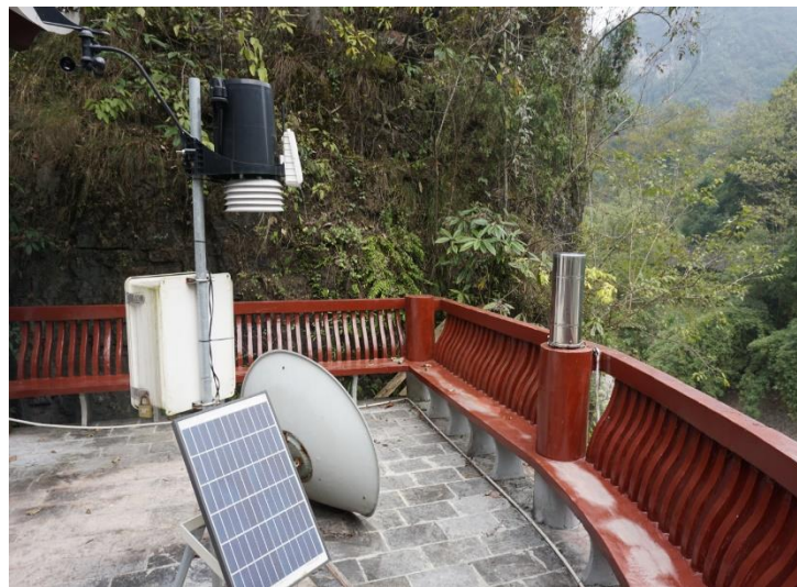
Figure 6 The hydrometeorological monitoring equipment in Shibing Karst
