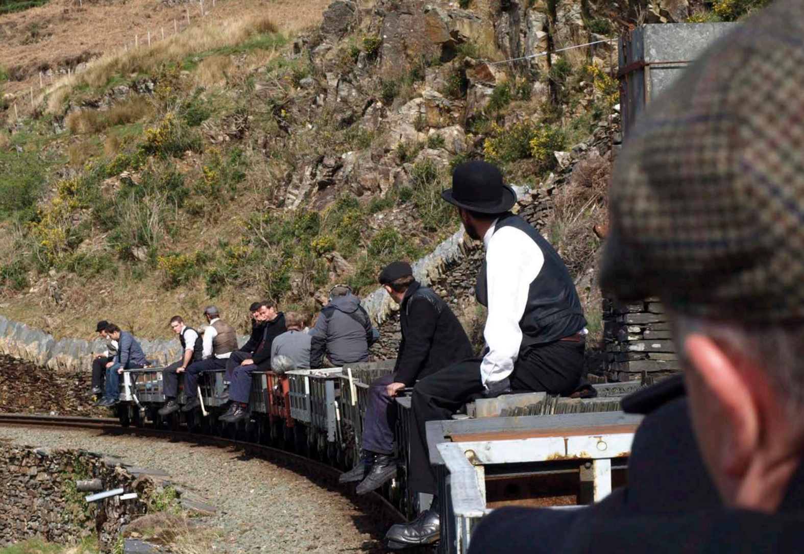
The Ffestiniog Railway runs demonstration gravity trains with its fleet of restored slate wagons, recreating the railway's operation from 1836 to 1940 © Ffestiniog and Welsh Highland Railways.
