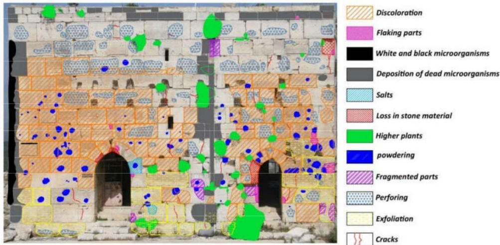
Figure 8 deterioration mapping of the external southern east façade of king's daughter tower
