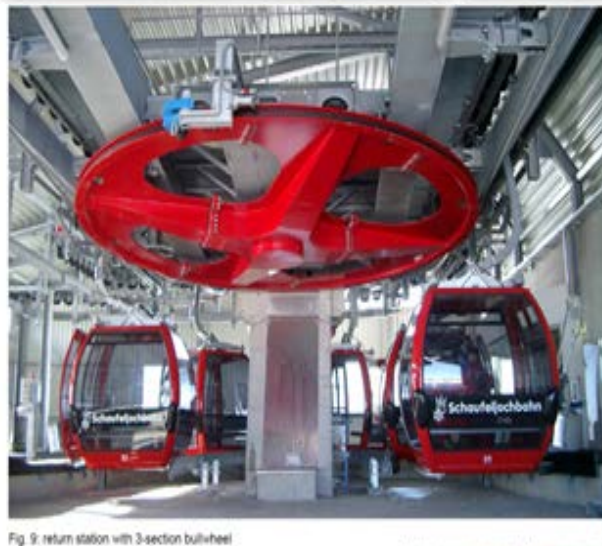
Fig. 9: return station with 3-section bullwheel
