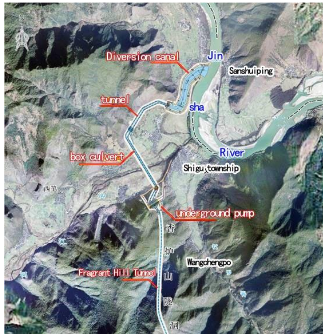
Figure 11: Schematic diagram of Shigu water diversion
