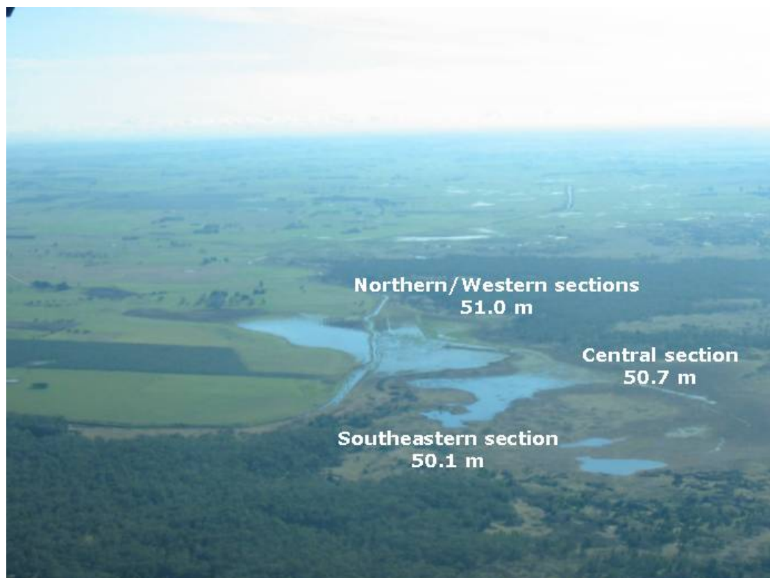
Figure 44. Aerial photograph taken in 2001 (date unknown) showing Lake water at three different levels. Levels determined from comparison with 2005 DEM. Photograph taken from Ruge (2004, p. 42), credited to Glenelg Hopkins CMA. The Northern and Western sections are hydraulically connected to the Drain, while the rest of the Lake is disconnected.
