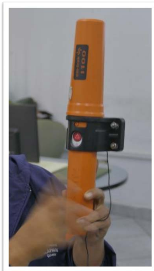
Picture 6 – Beacon provided by the GNP administration to small boats (Source: EMC21).
