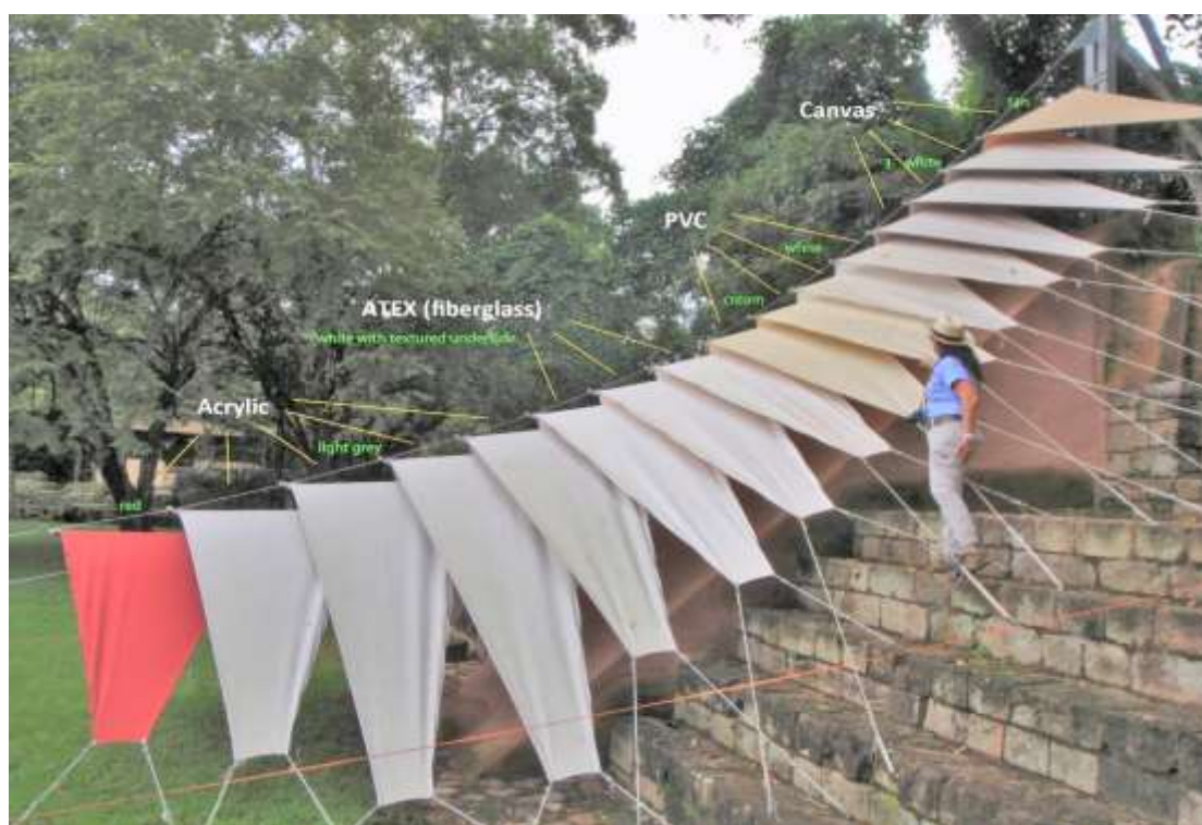
Figure 15: Prototype of the “Cascading Sails” protective structure for the Hieroglyphic Stairway
