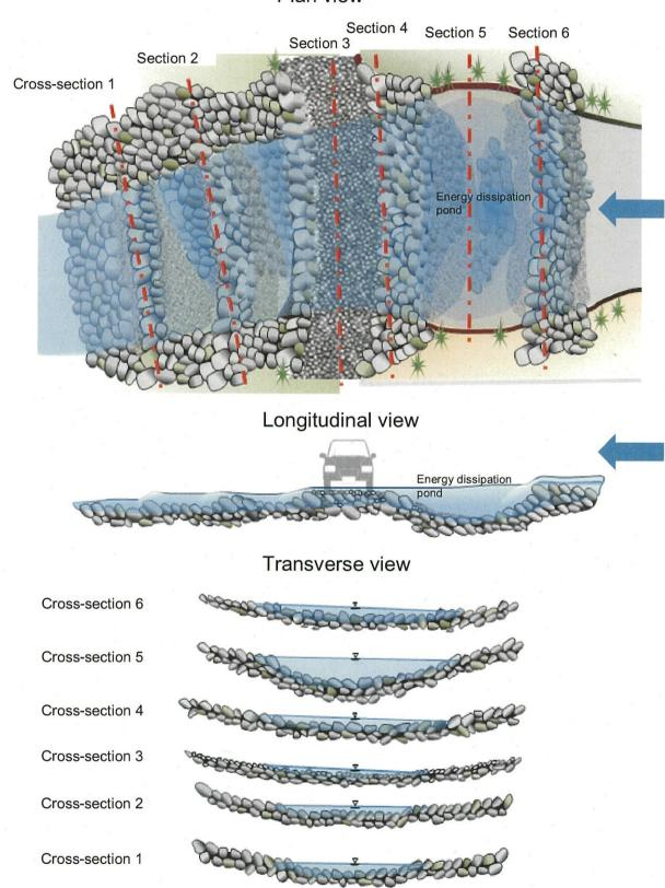
The upper and lower sides of the raised riverbedl will be protected by a 50-cm-wide stone riverbed sill. (The cross-section will be arch-shaped to avoid a sharp change in shape.)
