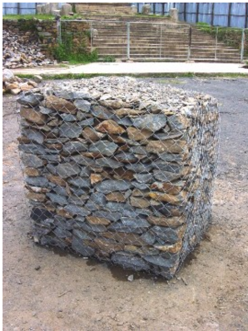
Sample of gabion for the construction of the temporary embankment
