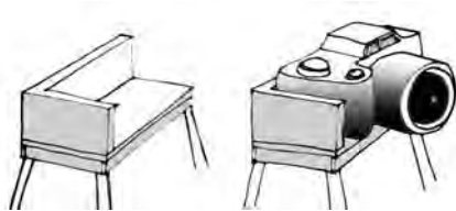
Type of permanent stand which is needed. The camera is not screwed to the foot, it is simply placed on top of it. This can be produced by local welding workshops.
