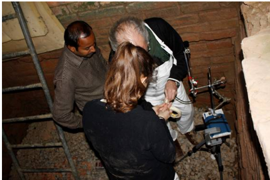
Water capillary absorbance Ashok Pillar
