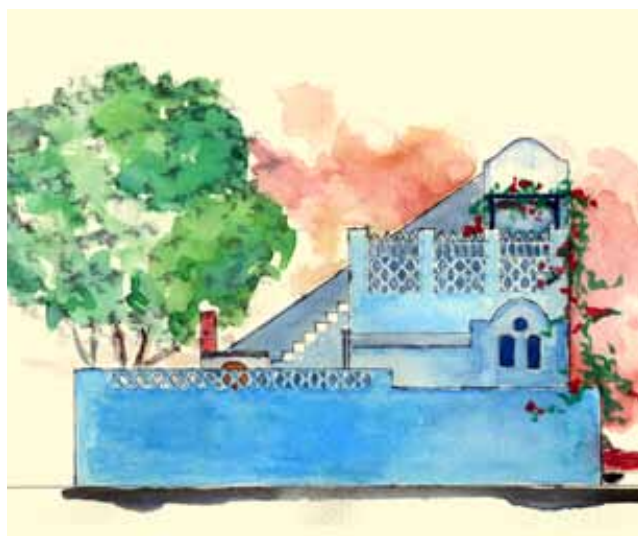
Figure 3: Eco-lodge prototype 'G' for Mr AbdAllah Schleifer, Tunness, Fayoum oasis. Egypt. 1992-93. Western façade rendering in watercolor (by Mr Seif El Rachidy) showing the multiple walled envelopes to the core space of the eco-lodge prototype. © Ahmad Hamid Architects
