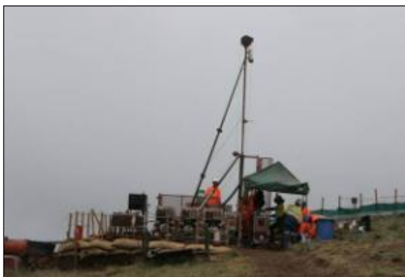
Photo 7 – Station mobile de carottage, concession SMFG (Source : EMC2I).
