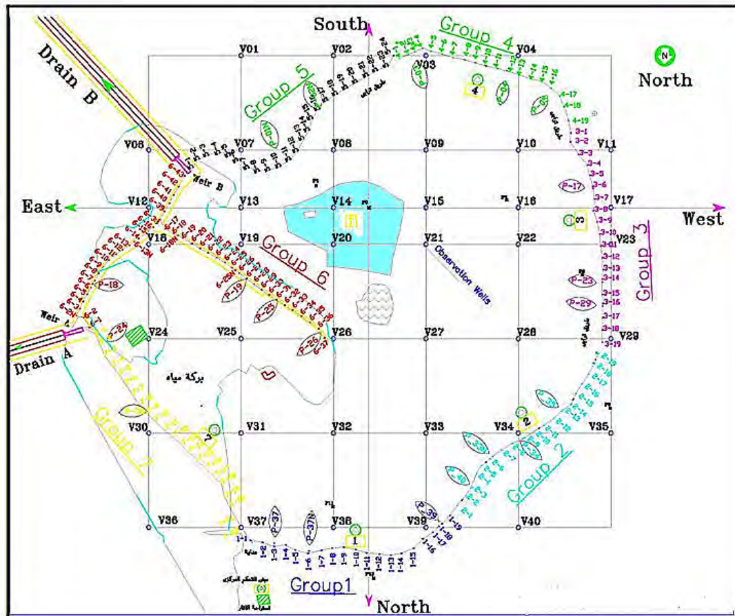
Figure 4 Implementation of the new project. The archaeological site (light blue area) is surrounded by 170 pumping wells, arranged in seven groups (1-1, 1-2.; 7-1, 7-2....). The water table is monitored at 40 observation wells (V1, ..., V 40). Water is conveyed to two open-air canals (Drain A, Drain B), which are connected to a main canal, about 30 km long, discharging in the Mediterranean Sea in the vicinity of Alexandria. [Document released by the Ministry of Culture]
