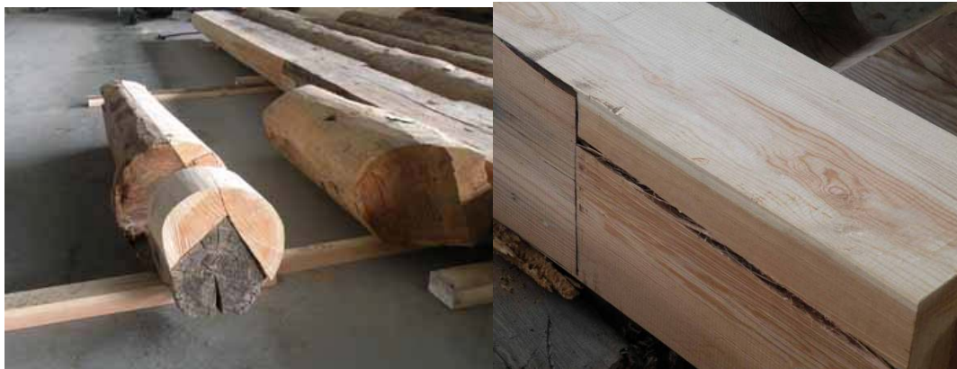
Figure 2 – Wood expands and contracts daily and yearly according to its structure. This contributes to the ultimate failure of glue joints which tend to be rigid.
