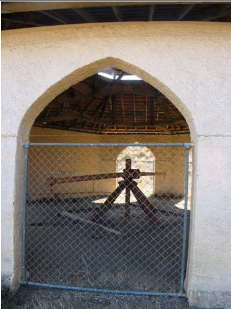
Timber hose pump and spar set in Tread Mill and modern cyclone wire fence
