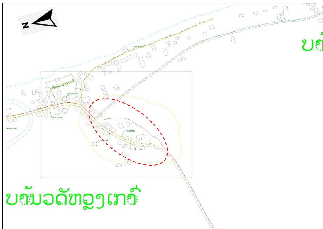
Figure 3 The channel's line has been changed once it passes the archaeological site to ensure that the properties would not be damaged.
