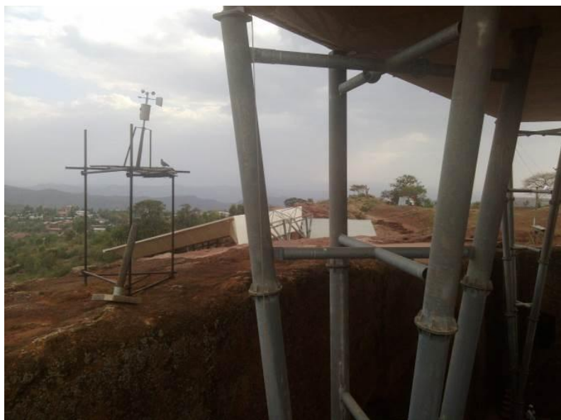
Figure 21 -Weather station not in use and now posing a visitor risk due to rotten planks on which it is mounted
