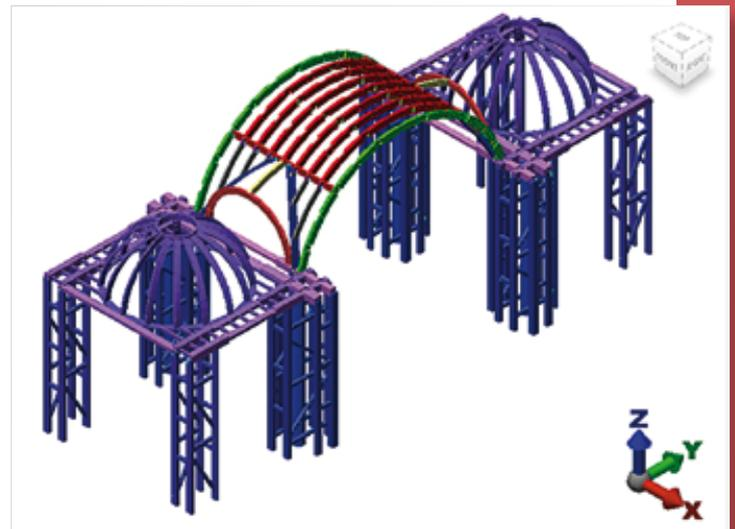
*Figure 11: Partial numerical model of a representative bay of the nave and side aisles of Ica Cathedral, where the most important timber joints are simulated using realistic stiffness values obtained during the experimental campaign performed by PUCP. © Image and model: Carina Fonseca Ferreira, UCL, The J. Paul Getty Trust, 2013*
