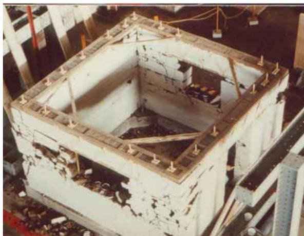
conducted in a new PUCP structural laboratory (Ottazzi *et al.*, 1989). Housing modules without roofs, with and without internal cane reinforcement, were tested according to the National Construction Regulations (MTC, 2000).
