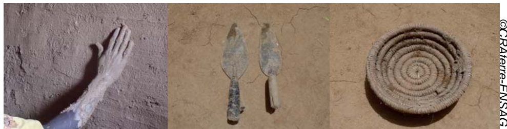
Earthen architecture tools and methods used in Djenné, October 2011
